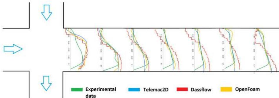
Figure 4 Horizontal velocity profiles downstream to the junction C-4
