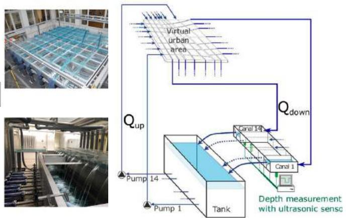
Figure 2 Scheme of the water cycle in the experimental model
