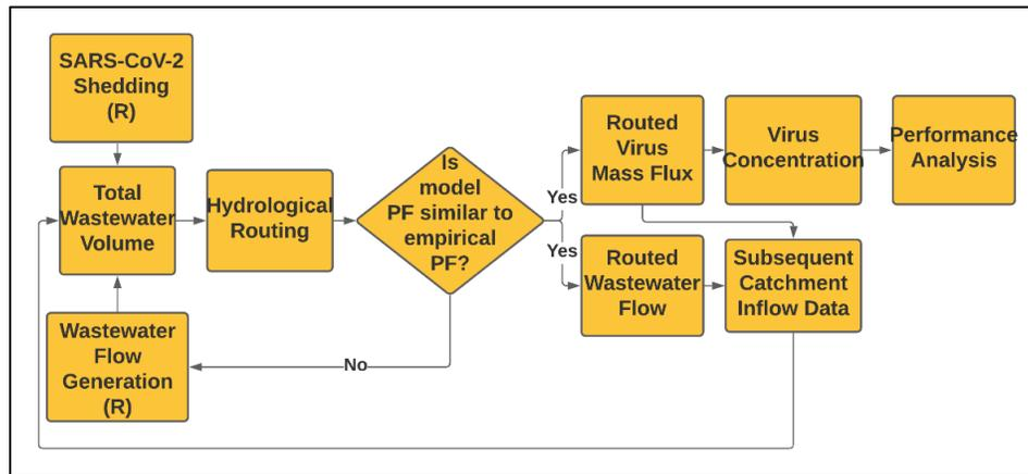
**Figure 1.** Flowchart of the model for a single catchment scale, where (R) denotes randomised input parameter.
