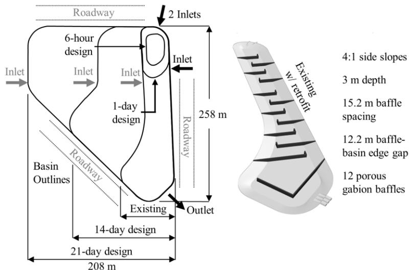
**Figure 1.** Dimensioned outline of modeled basins and isometric view of the retrofitted existing basin
