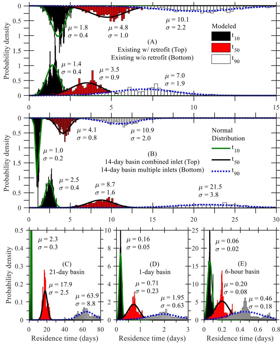
**Figure 2.** Frequency distributions of modeled wet season residence time distribution (RTD) metrics.  $t_x$  represents the elapsed time at which x percent of elution has occurred. Fitted normal distributions are plotted alongside modeled data with mean ( $\mu$ ) and standard deviation ( $\sigma$ ) values provided. Results shown for the CFD with implicit solution stepwise steady (IS3) model.
