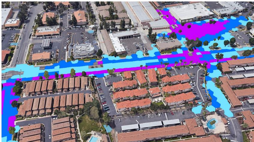
**Figure 2.** Inundation extents along Winter Gardens Boulevard in the proposed condition after upgrading storm drain backbone during the 100-year 24-hour storm event.
