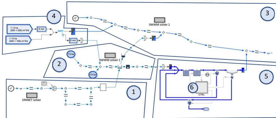
**Figure 1.** Multi-Solve simulator modelling different components of an urban water system using different solvers
