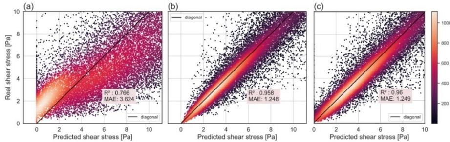
**Figure 1.** Results of the ML regression algorithms for the shear stress in the range of 0 – 10 Pa (a) linear regression (b) random forest (c) neural networks. The colours indicate the number of data points.
