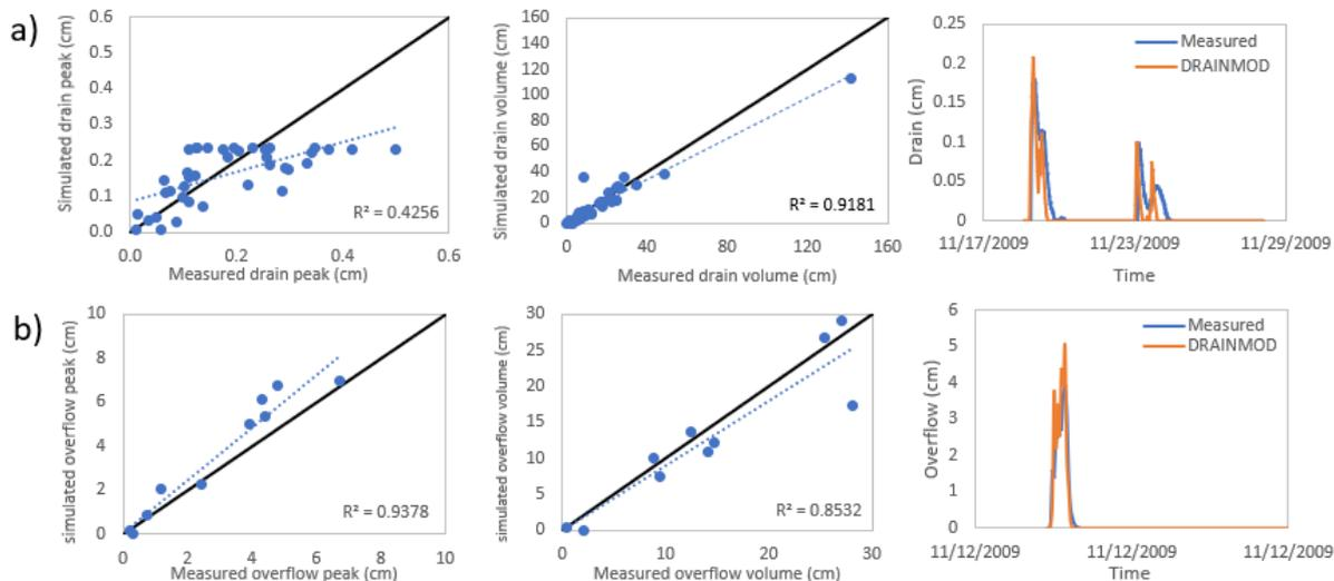
**Figure 1.** DRAINMOD-Urban performance in the post-repair 0.9-m media depth cell. a) measured versus simulated drain event peak (left), volume (middle), and hydrograph (right). b) measured versus simulated overflow event peak (left), volume (middle), and hydrograph (right)
