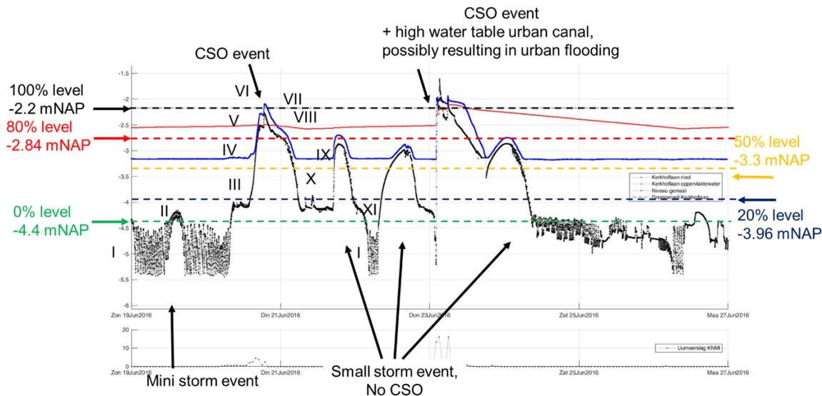
**Figure 2.** Typical events (DWF, mini storm event, small storm event and very large storm events) and filling degree thresholds determining the stage of the RTC system. NAP indicates mean sea level. Horizontal coloured lines indicates the water levels that determine the stage of the sewer system. The stage determines the RTC-objective which gets priority.
