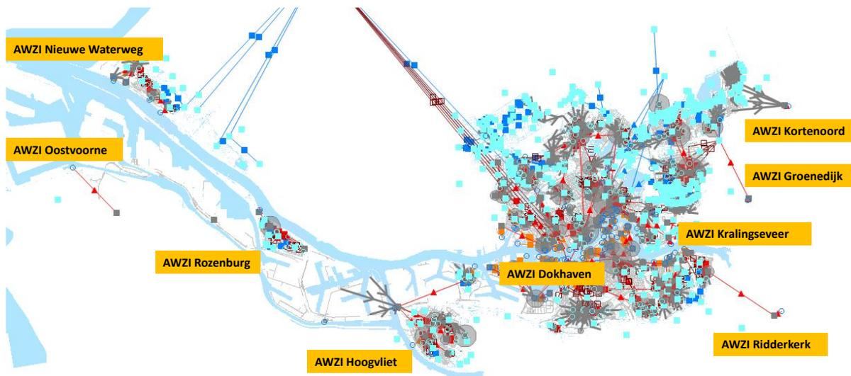
Figure 1. Sewer model of Rotterdam sewer system. The yellow blocks indicate the location of the downstream WWTPs.
