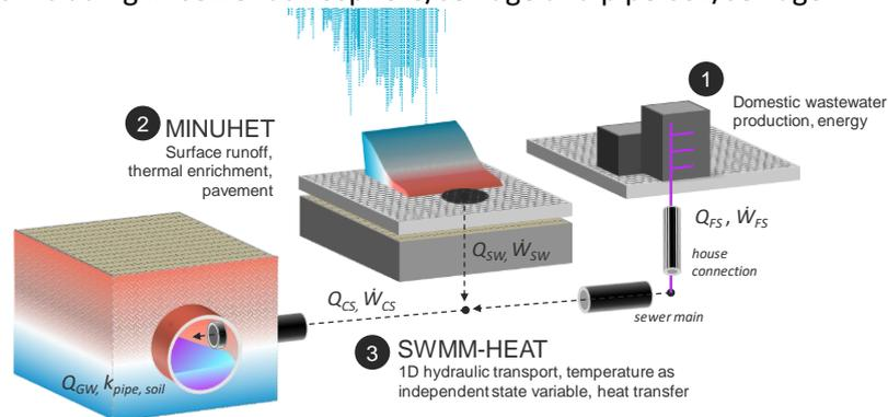
The suggested approach requires a careful treatment of the information provided by numerous sources. Figure 2 shows a scheme of the dataflow adopted to inform the SWMM-HEAT tool: flow and temperature time series from runoff and wastewater produced by households are mixed using the alligation method, while groundwater infiltration patterns are provided in the SWMM-HEAT input file. Once the routing simulation starts, an internal module in SWMM-HEAT mixes the thermal-hydraulic flows accordingly.
