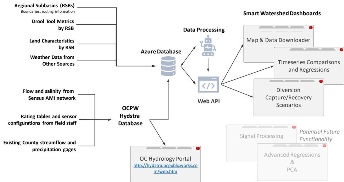
**Figure 1.** Architecture Schematic of Data Pipeline and Federation System
