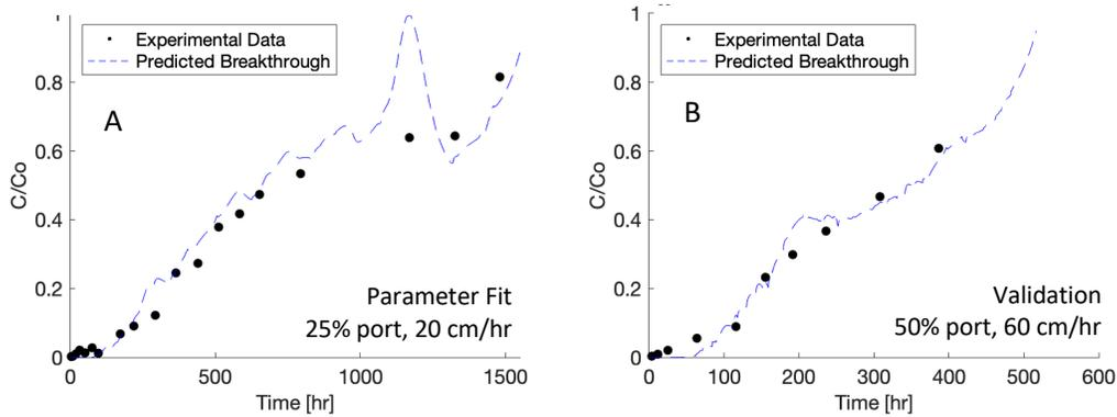
**Figure 1. (A)** Model fit to breakthrough data for Atrazine at the 25% sample port for the 20cm/hr experiment. **(B)** Model prediction validation for Atrazine at the 50% sample port for the 60 cm/hr experiment.
