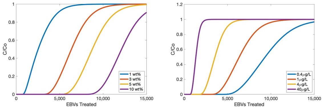
**Figure 2.** Predicted Atrazine breakthrough in 1-meter biochar-amended columns operated at 20 cm/hr with (unless specified otherwise) 3% wt biochar and an influent concentration of 1  $\mu\text{g/L}$ .
