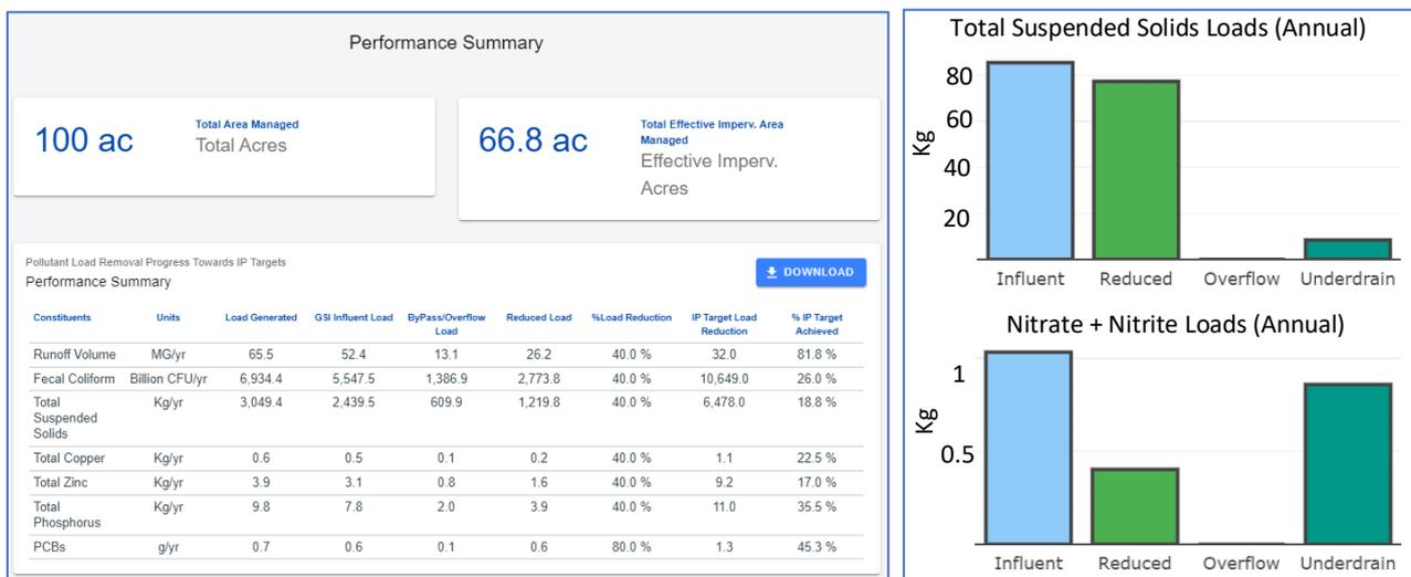
**Figure 2.** Example performance summary of the PPET for a conceptual bioretention system (left). Graphical output of scaled annual influent, overflow, and underdrain loads of total suspended solids and nitrate + nitrite based on monitoring data using the MRLC tool. Reduced loads are those infiltrated or retained by the bioretention systems.
