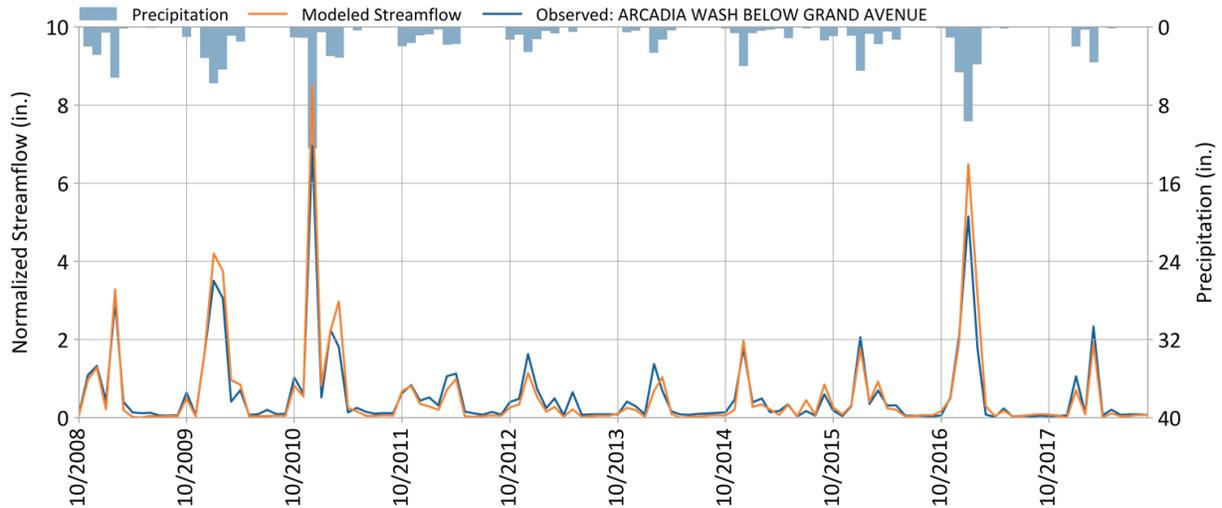
**Figure 3.** Observed compared to Model Flow at Arcadia Wash below Grand Avenue from October 2008 to October 2018.
