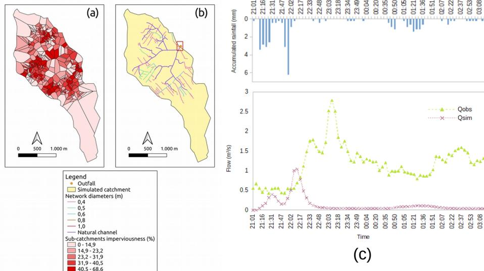
**Figure 2.** (a) The sub-catchments imperviousness percentages, obtained from buildings and traffic zones polygons; (b) The simulated catchment and the pipes and channels diameter; (c) The observed (Qobs) and the simulated (Qsim) hydrograms for 1<sup>st</sup> Jan 2018 precipitation event.
