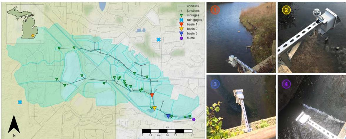
**Figure 1.** Study area with sensors placed at four sites on the stormwater system mainstem.
