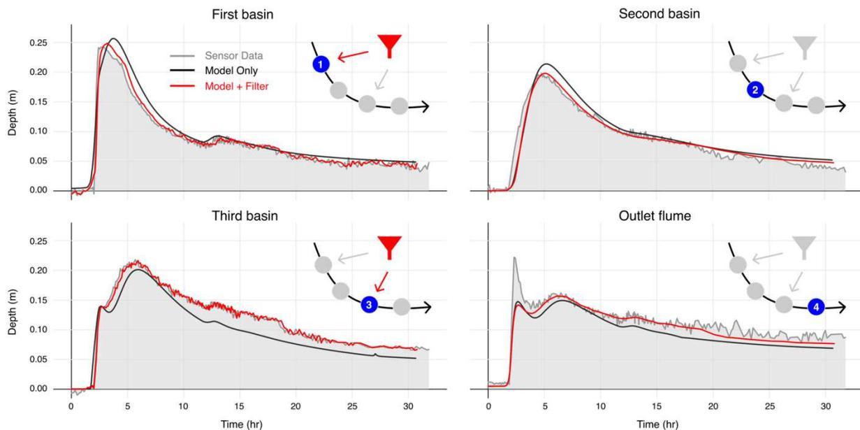
**Figure 2.** Validation of Kalman filter using a holdout assessment. (Left): Depth hydrographs at sites 1 and 3, where the Kalman filter is applied. (Right): Depth hydrographs at locations where Kalman filter was not applied. The Kalman filter reduces error at both holdout sites.
