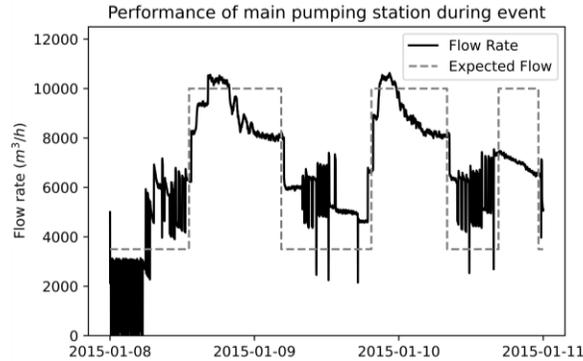
Figure 2 - Difference between expected flow and performed flow by main pumping station
