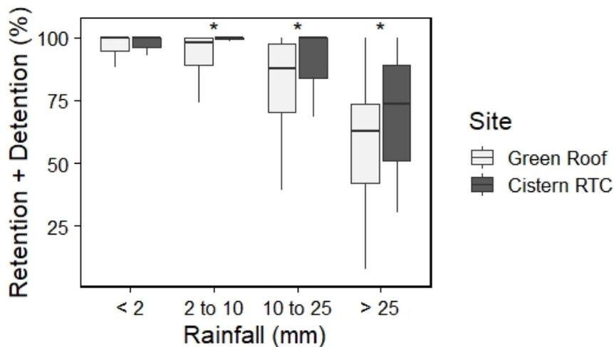
**Figure 3.** Total on-site retention + detention for different storm sizes. The \* at the top denote groups where the difference between Cistern RTC and Green Roof was statistically significant ( $p < 0.05$ ).
