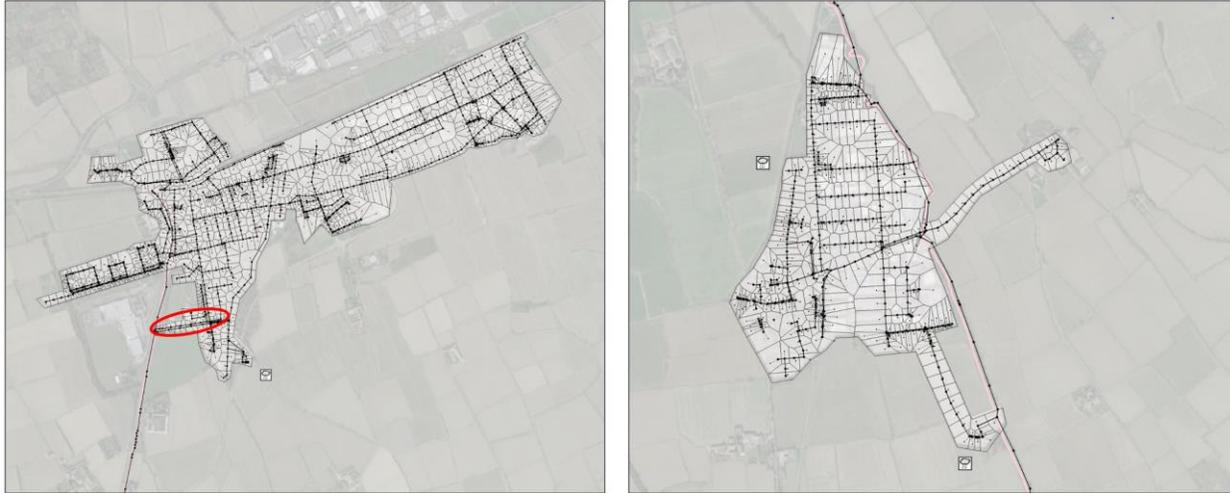
**Figure 2.** Model geometry in SWMM: visualization of the urban drainage system with highlighted CSO number 416.
