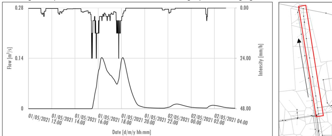
**Figure 3.** Rainfall measured at P\_GAG01 and simulated hydrograph in CSO number 416 for the event of 1 May 2021.
