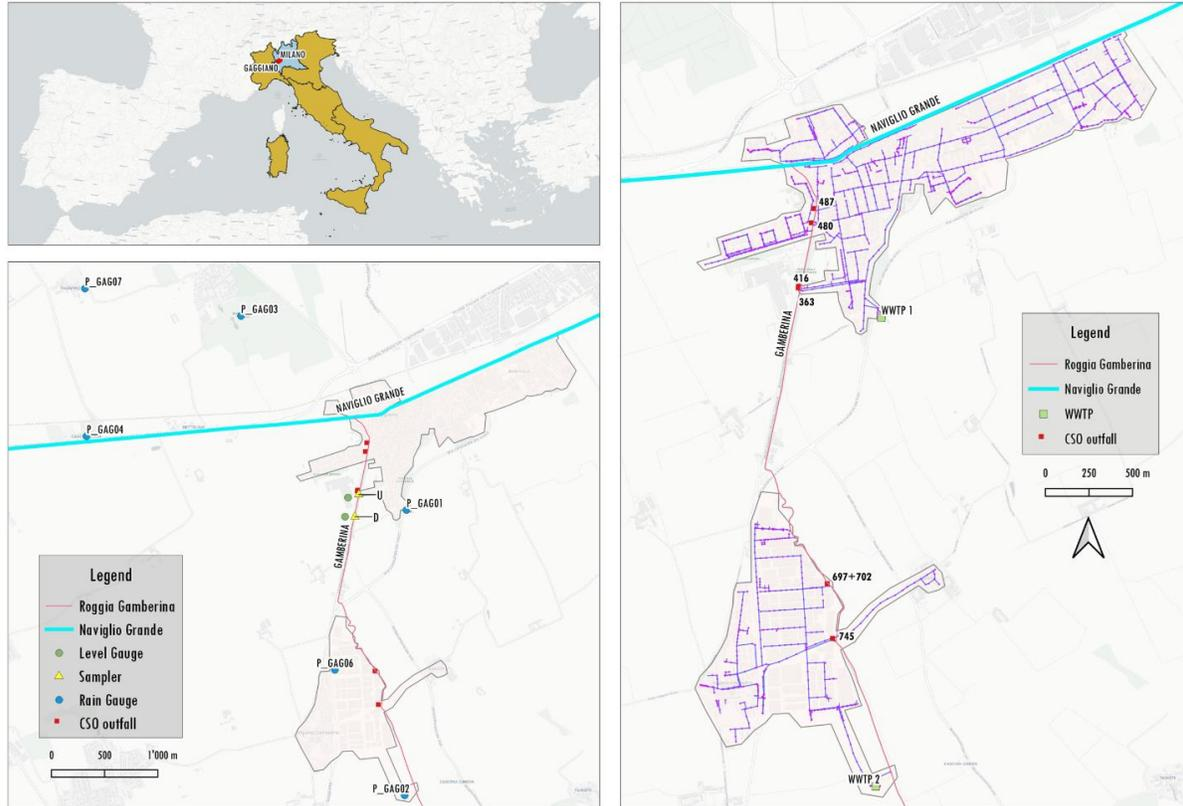
Figure 1. Case study domain: sewer network and measuring system collocation.
