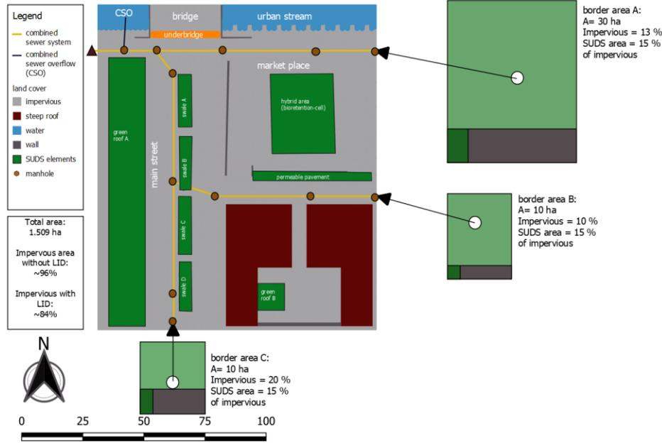
Figure 1: The Character of the virtual urban catchment area ( A = 1.509 ha) with three border areas (border area A: 30 ha, border area B and C: 10 ha) including the places of the SUDS assets (green roof, bio-retention cell, permeable pavement and swales)
