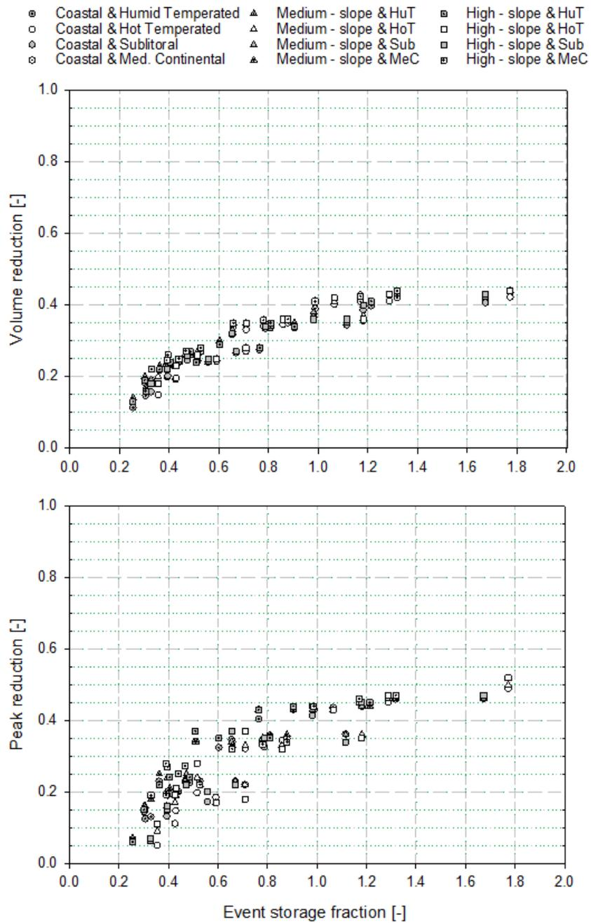
**Figure 1.** Volume and peak reduction indexes plotted versus the event storage fraction simulated for the three drainage network catchment typologies (Coastal, Medium-slope; High-Slope) according to the four precipitation regimes (Humid tempered, Hot tempered, Sublitoral and Mediterranean continental).
