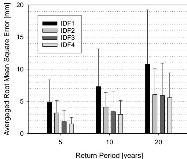
**Figure 1.** Comparison between the averaged Root Mean Square values of the different IDF equations assessed for the return period equal to 5, 10 and 20 years. The standard deviation associated with each estimated error is also reported.
