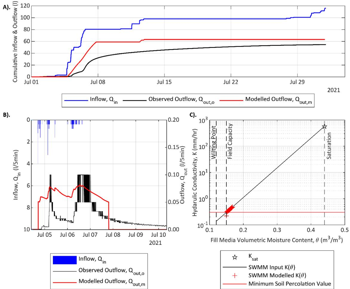
**Figure 1. A).** Cumulative Inflow and Outflow for Lysimeter 7b for July 2021. **B).** Inflow and Outflow for Lysimeter 7b from July 4<sup>th</sup> to 11<sup>th</sup>. **C).** Hydraulic Conductivity Function used in the SWMM model
