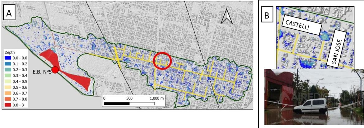
Figure 3. A: Waterlogging after 12 hours simulation for the Reference Scenario. B: simulated waterlogging vs. observed waterlogging for April 10th 2021 storm event. Castellí Street - San José Street intersection.
