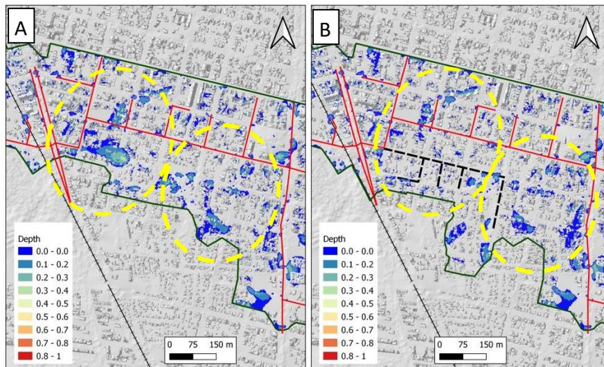
Figure 4. Effect of the designed J.P. López conduits system on the runoff pattern. A: Reference Scenario; B: Intervention Scenario.
