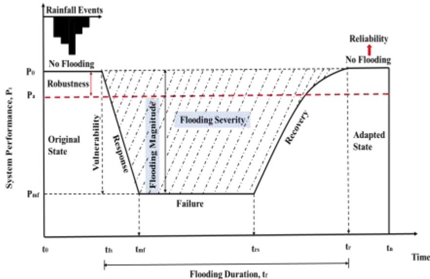
**Figure 1.** The system performance curve of an urban drainage system for a failure-causing rainfall event (The  $t_o$  is the time of occurrence of storms; The  $t_{fs}$  is the flood starting time; The  $t_{mf}$  is the starting time of maximum failure; The  $t_{rs}$  is the ending time of maximum failure; The  $t_r$  is the recovery ending time; The  $t_f$  is the flooding duration; The  $t_n$  is the total simulation time). This figure is adopted from previous work (Li et al., 2021)
