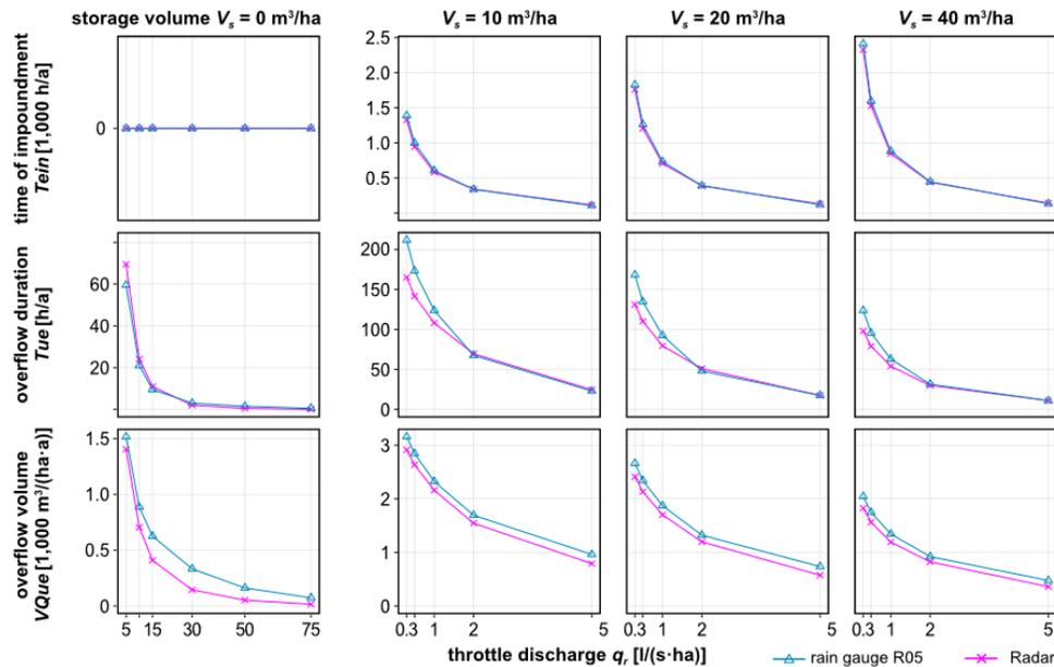
Figure 2. Results of precipitation-runoff simulations for generated long-term time-series data.
