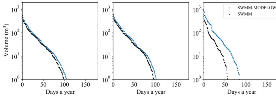
**Figure 2.** Frequency analysis of daily peak volumes at the three of the six critical zones. Results obtained with the coupled SWMM-MODFLOW and the uncoupled SWMM models are presented
