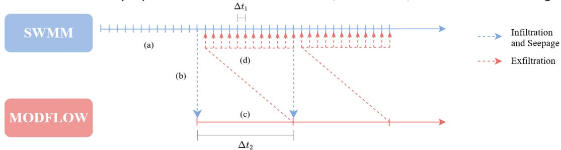
**Figure 1:** Temporal data exchange structure. (a) Surface rainfall-runoff is simulated using SWMM at a time step  $\Delta t_1$ . (b) The aggregated infiltration and seepage are transferred to the MODFLOW model as recharge. (c) Groundwater is simulated using MODFLOW at a time step  $\Delta t_2$ . (d) Drained water from MODFLOW is integrated as exfiltration at a constant rate back to SWMM.
