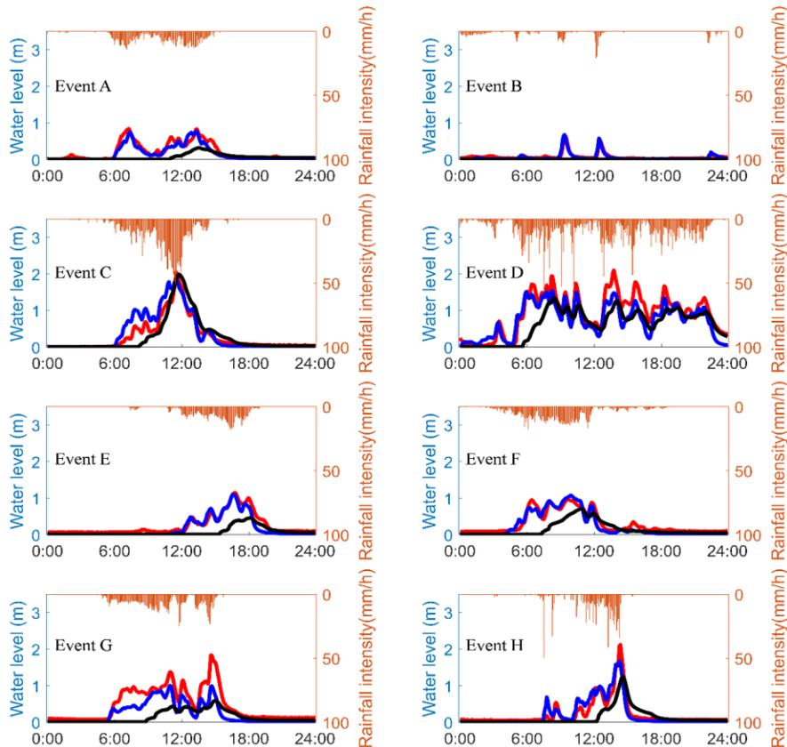
**Figure 3.** Time series of measured and simulated water level of 8 rainfall events. Red line: measurement; blue line: simulation with surface water discharge approach; black line: simulation without surface water discharge approach.
