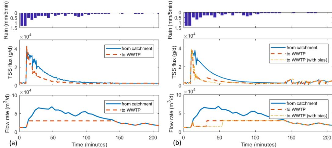
**Figure 1:** Illustration of the simulation results of (a) the reference scenario and (b) the optimal scenario on a low intensity rain event. On the right figures, results of the scenario with a positive bias are represented by the orange dash-dot line.
