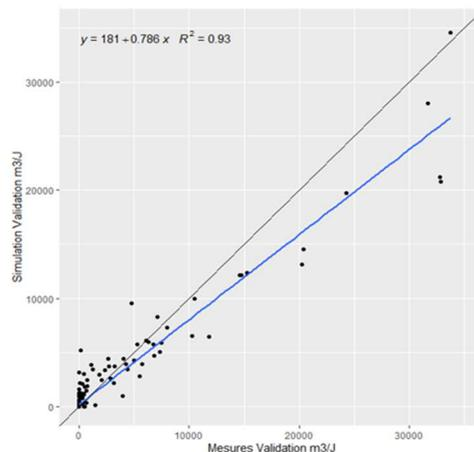
**Figure 1.** Simulated daily discharged volumes as a function of the measured daily discharged volumes, for the validation period (2018). The linear regressions, their equations as well as the R2 are plotted on the graphs.
