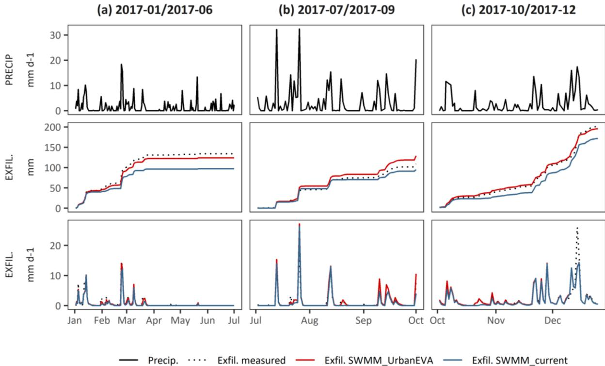
**Figure 1.** Measured and modelled exfiltration for green roof “FHZ”. Plotted periods are (a) calibration period and (b)/(c) two validation periods.
