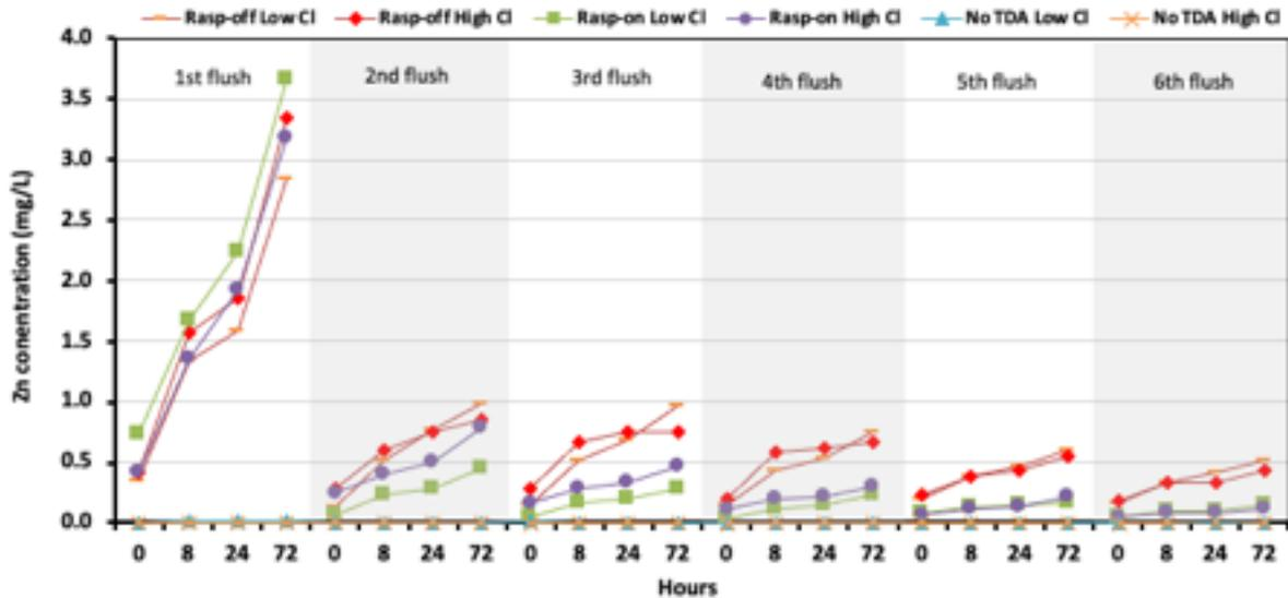
Figure 2. Zn concentration using phosphate buffer over multiple flushes.
