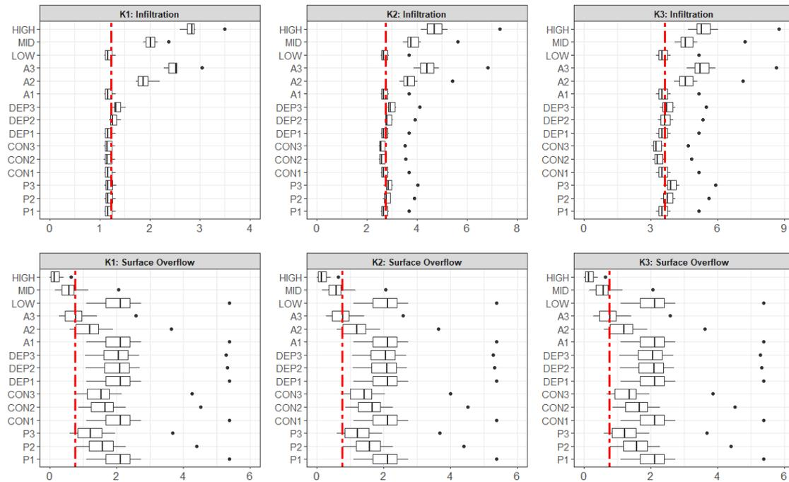
**Figure 1.** Boxplots depicting annual infiltration and surface overflow volumes (1000 m<sup>3</sup>/yr) from simulations of ten future (2040-2044) climate projections using various design configurations under three underlying soil conditions (K1: clay; K2: clay loam; K3: sandy loam). Performance under current standards and 2010-2014 climate data shown in dashed, vertical red lines.
