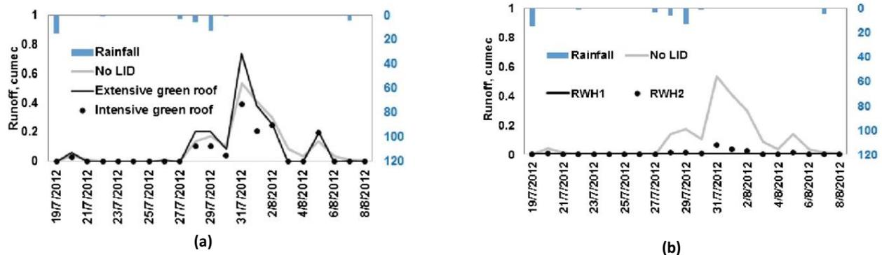
**Figure 3.** Event-based analysis of runoff from Velachery catchments for rainfall events with fewer than 10 antecedent dry days. Plots compare runoff from urbanized scenario with (a) green roof (b) rain water harvesting structures RWH1 and RWH2
