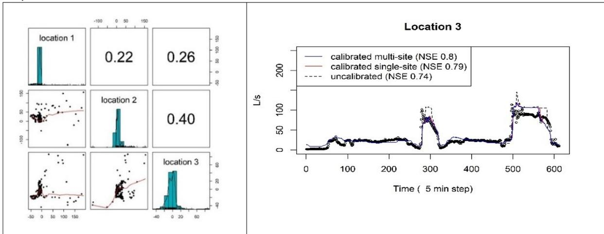
Figure 2a: Correlation between model errors. While one expects a strong correlation between *observations* (flow in L/s) at adjacent locations, we find there is only weak correlation between *model errors* (in L/s). Therefore we assume the errors to be spatially independent during inference. 2b: Model performance (here shown at location 3) does not show any significant improvements when parameters inferred using data from multiple locations.
