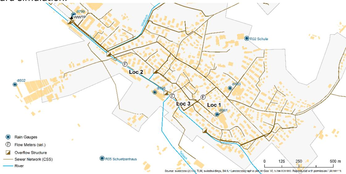
Figure 1: Layout of the case study in Fehraltorf, Switzerland. Sewer network, rain gauges and corresponding flow monitors (loc 1, loc 2, loc 3) are indicated.
